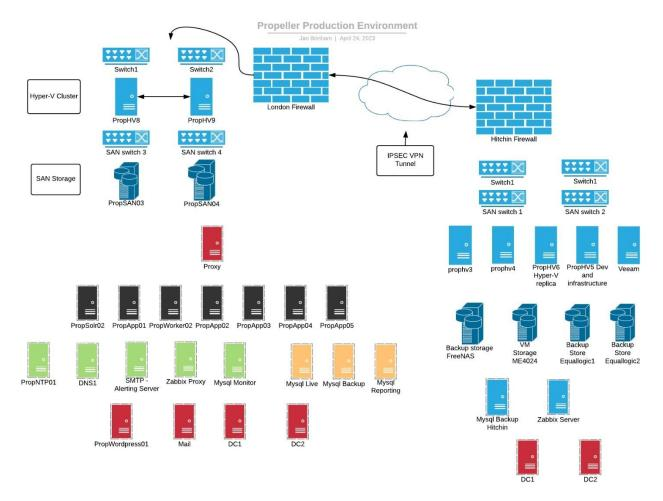
The primary array – This network of computers, switches, firewalls and hard storage units make up the dayto-day system that delivers the company's application hosting services.
